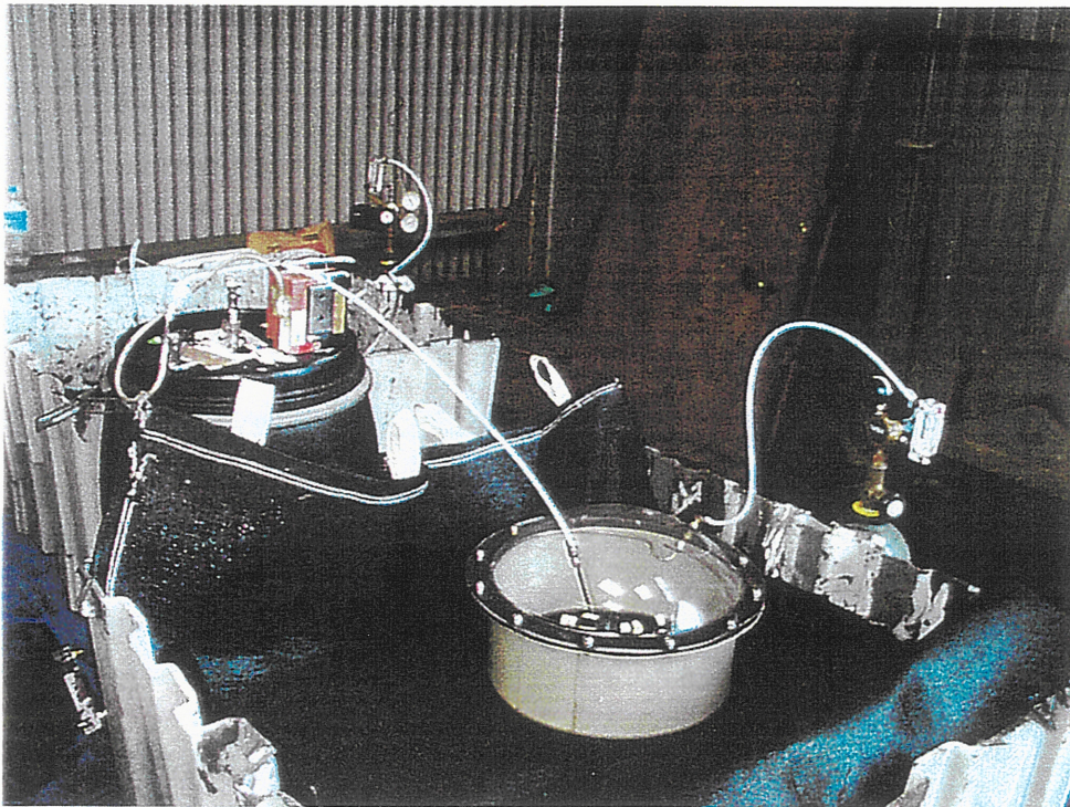
Photo 3 VOCs and PAHs Sampling from the odour pen with geotextile bag
