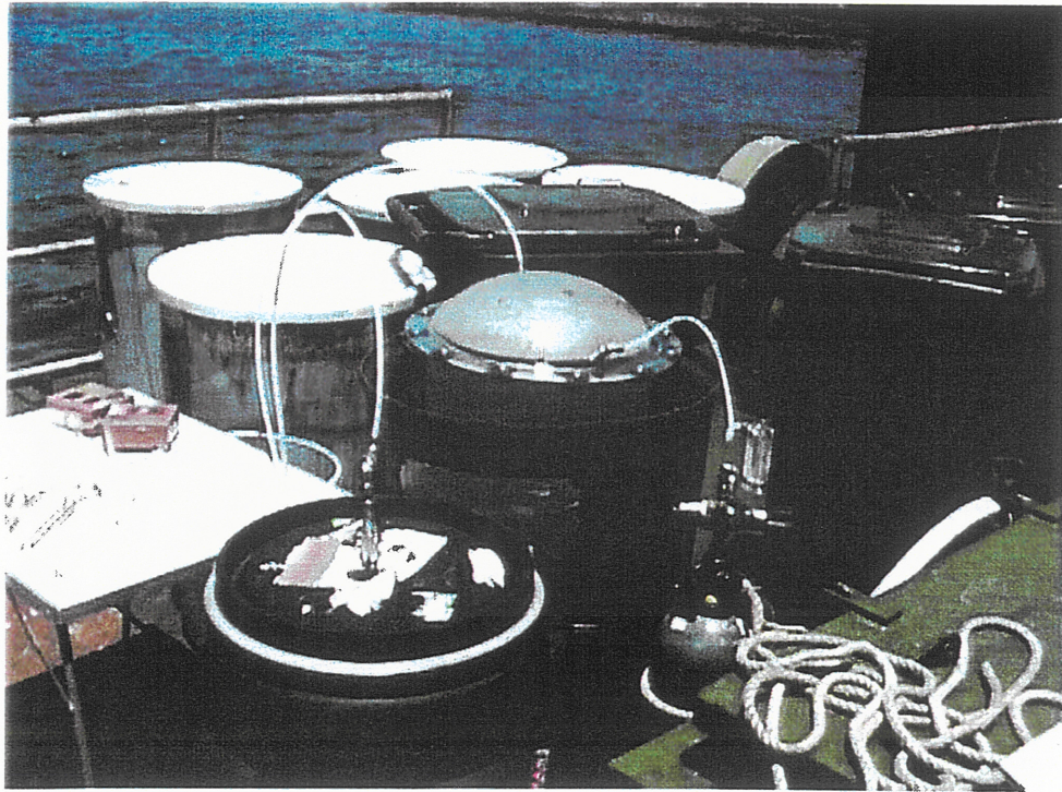
Photo 5 Odour sampling from the barrel on the dredging barge
