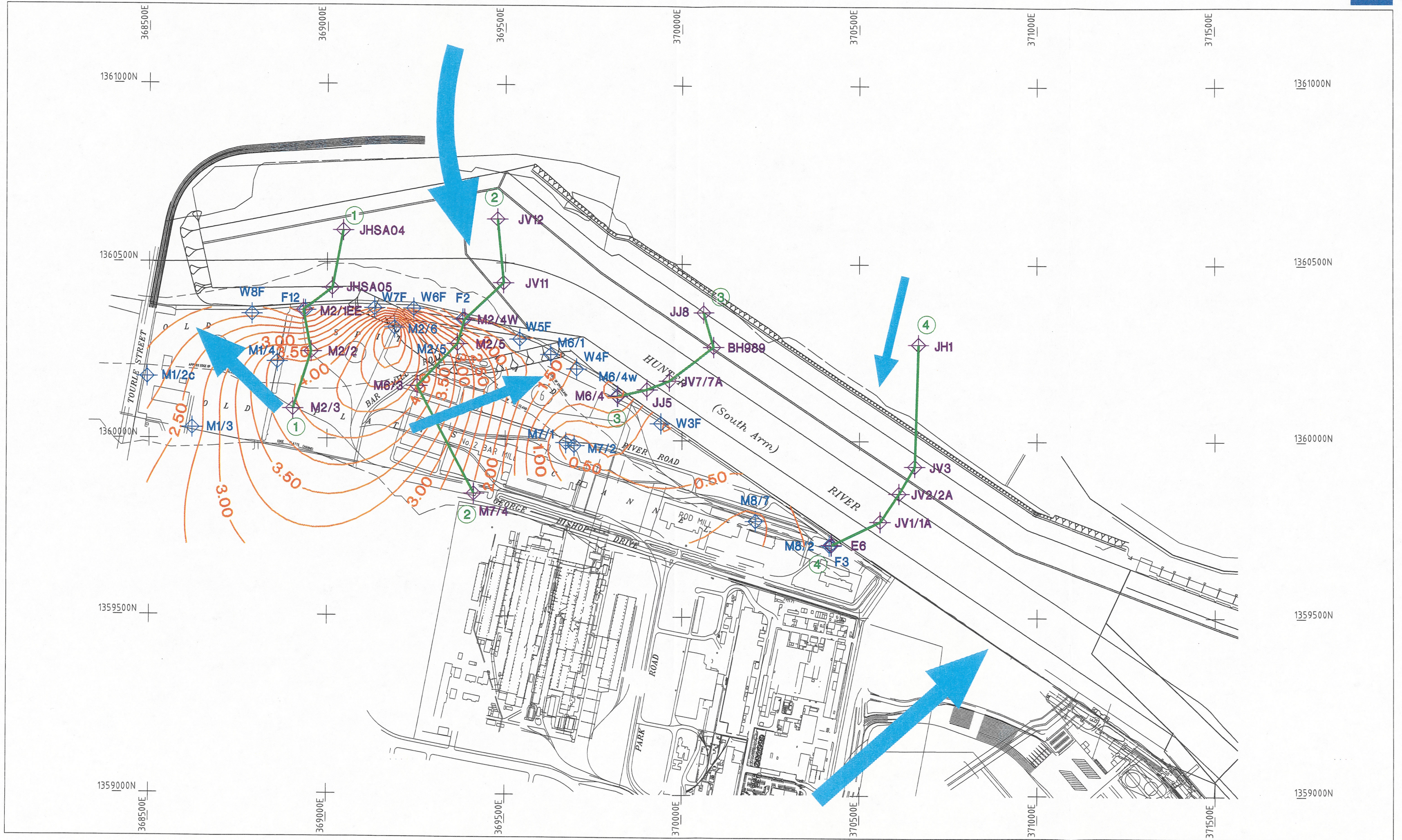
FIGURE HYDRO.1 AVERAGE INFERRED GROUNDWATER LEVEL CONTOURS (MARCH 2002 TO JULY 2002) IN THE VICINITY OF THE PROPOSED SHORTLAND SWING BASIN - FILL AQUIFER. LOCATION OF CONCEPTUAL HYDROGEOLOGICAL CROSS SECTIONS
