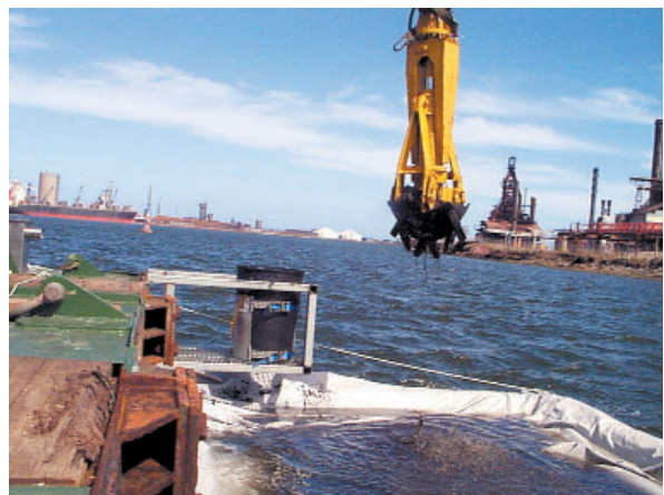
Plate 17.4 Hydrogen sulphate sampling from the odour pen with geobag
