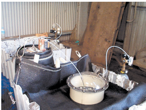
Plate 17.3 Volatile organic compounds and polycyclic hydrocarbons, sampling from the odour pen with geobag
