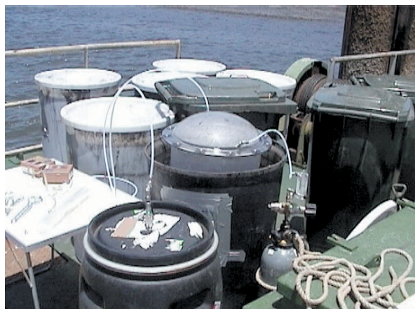
Plate 17.5 Odour sampling from the bucket on the dredging barge
