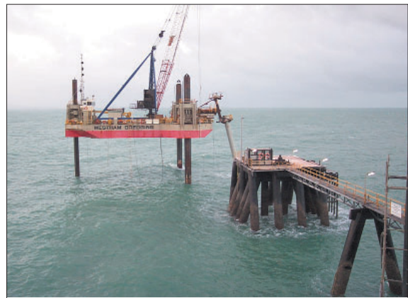
Plate 6.10 Self elevation platforms
