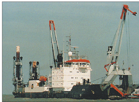
Plate 6.8 Large cutter suction dredge
