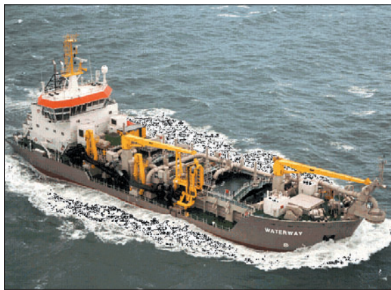
Plate 6.7 Small trailing suction hopper dredge
