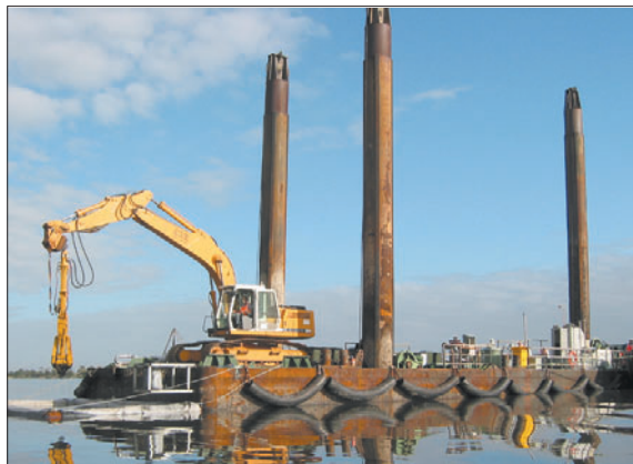
Plate 6.3 Medium sized backhoe dredge
