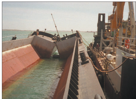
Plate 6.6 Split hopper barge
