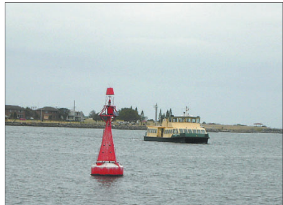
Plate 6.2 Example of navigation aids - floating bouy
