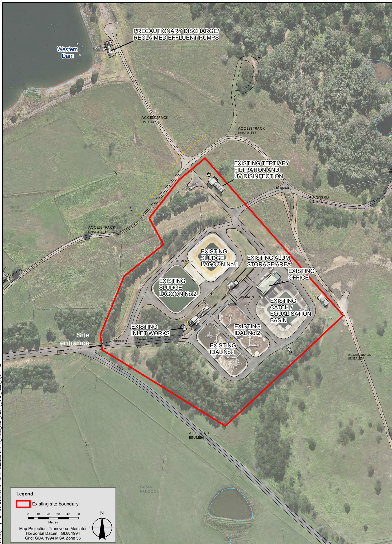
Figure 2.2 Picton WRP – existing facilities
